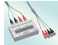
TEST FIXTURE 9261-10 Cable length 1 m (3.28 ft), DC to 8 MHz, impedance characteristics of 50 Ω, 4-terminal pair configuration, measurable conductor diameter: φ0.3 (0.01 in) to 1.5 mm (0.06 in)
