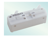
SMD TEST FIXTURE 9677 Direct connection type, For measuring SMDs with electrodes on the side; DC to 120 MHz, test sample dimensions: 3.5 mm ±0.5 mm (0.14 in ±0.02 in)
