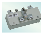
SMD TEST FIXTURE 9699 Direct connection type, For measuring SMDs with electrodes on the bottom; DC to 120 MHz, test sample dimensions: 1.0 mm (0.04 in) to 4.0 mm (0.16 in) wide, max. 1.5 mm (0.06 in) high
