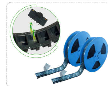
SMT and THR process Tape and reel package can be used for SMT and THR process to meet automated production
