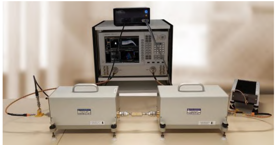
Pulsed DC and RF Load Pull bench architecture
