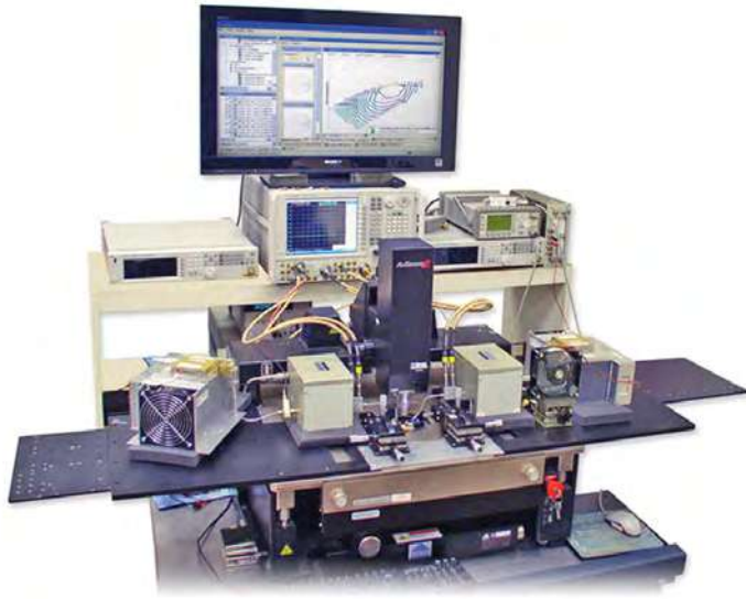
Hybrid-Active Load Pull at 30–50 GHz
